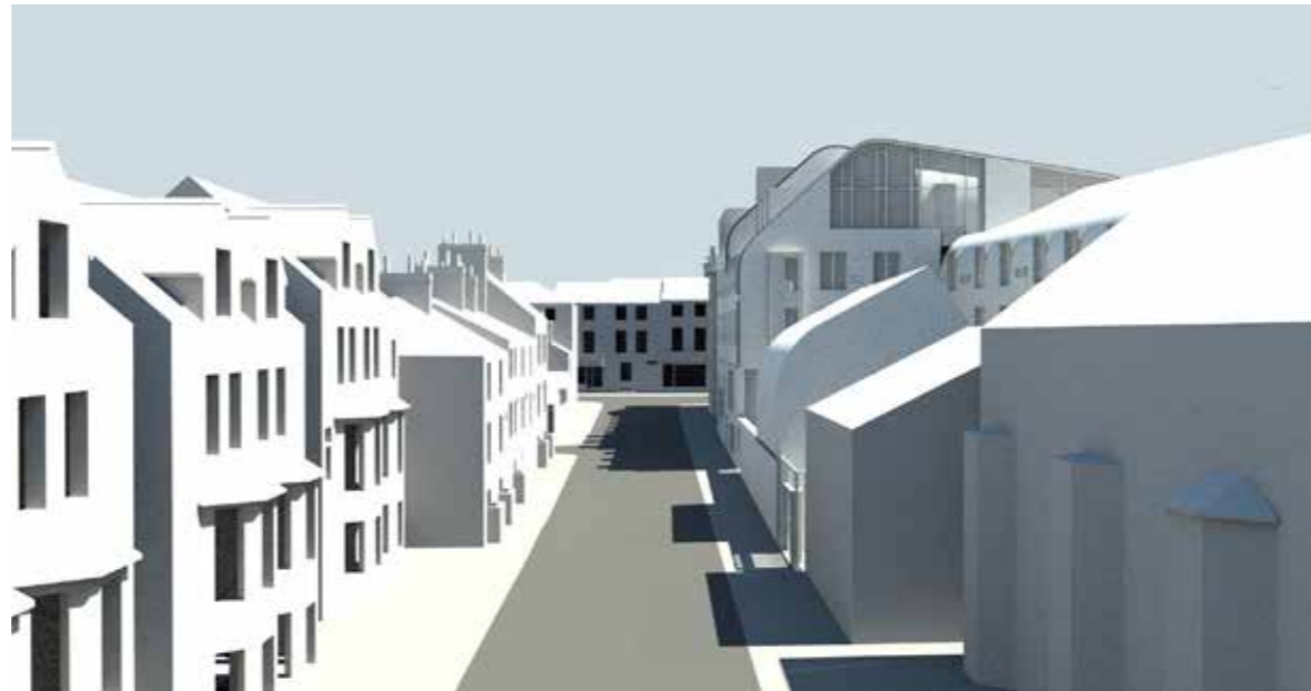
Diagram 01- Worcester Place Shadow Study Illustrates the shadows cast across Worcester Place during the summer solstice.
